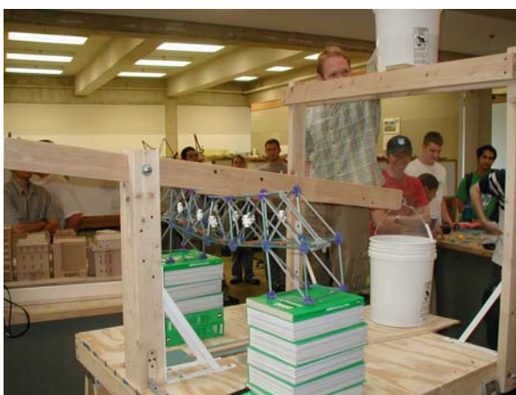
Figure 6. K'NEX beam loaded by cantilever arm with sand bucket filled from upper bucket. Lateral-torsional buckling clearly evident as failure mode (lower image).
