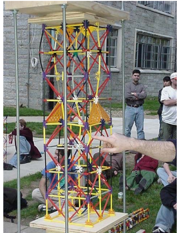
Figure 8. K’NEX column load test. Note Buckling of various rod members.
