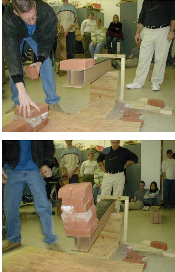
Figure 16. Test loading of cantilevered corrugated cardboard beam
