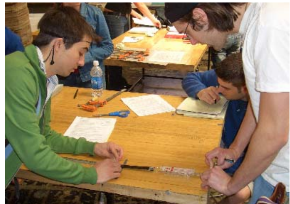
Figure 1. Elasticity lab using strips from plastic bags
