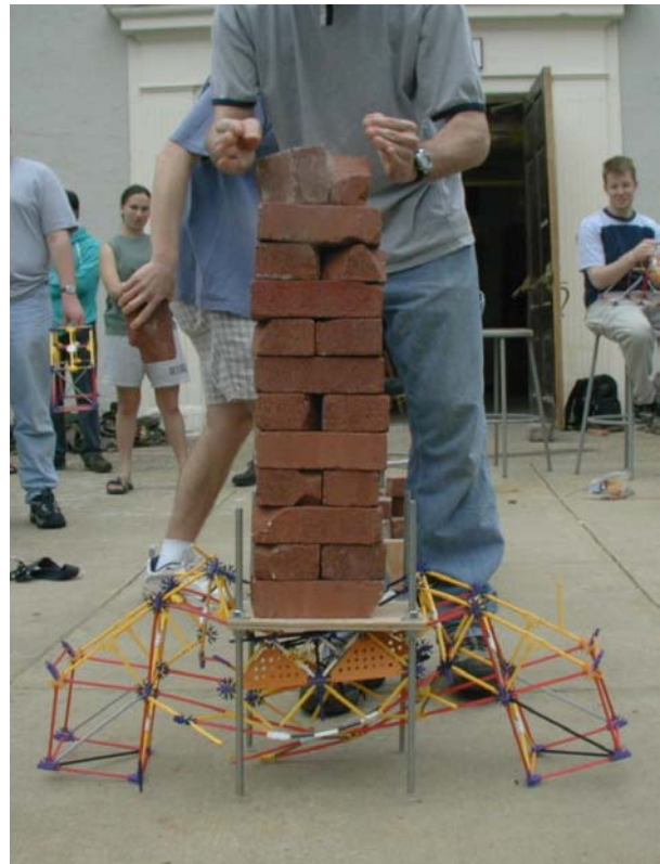
Figure 5 Bottom chord tension failure of K’NEX truss loaded with approximately 120 pounds of bricks.
