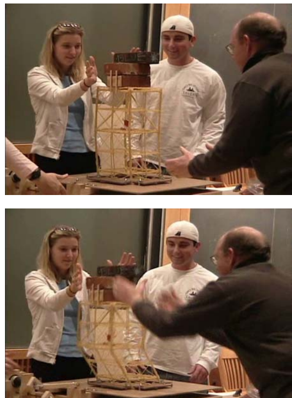
Figure 12. Soft story failure of pasta tower in shaker table test
